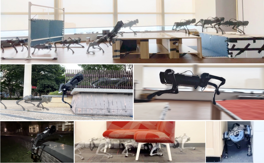
Figure 1: We present a framework for learning parkour skills on low-cost robots. Our end-to-end vision-based parkour learning system enable the robot to climb high obstacles, leap over large gaps, crawl beneath low barriers, squeeze through thin slits and run. Videos are on the project website .
